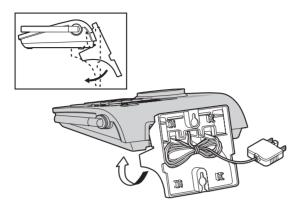
**4** Drive the screws (not included) into the wall using the wall mount template (see below) as a guide. Mount the unit and slide it down into position. Connect the AC adaptor and telephone line cord to their respective outlets. Raise the antennas.
